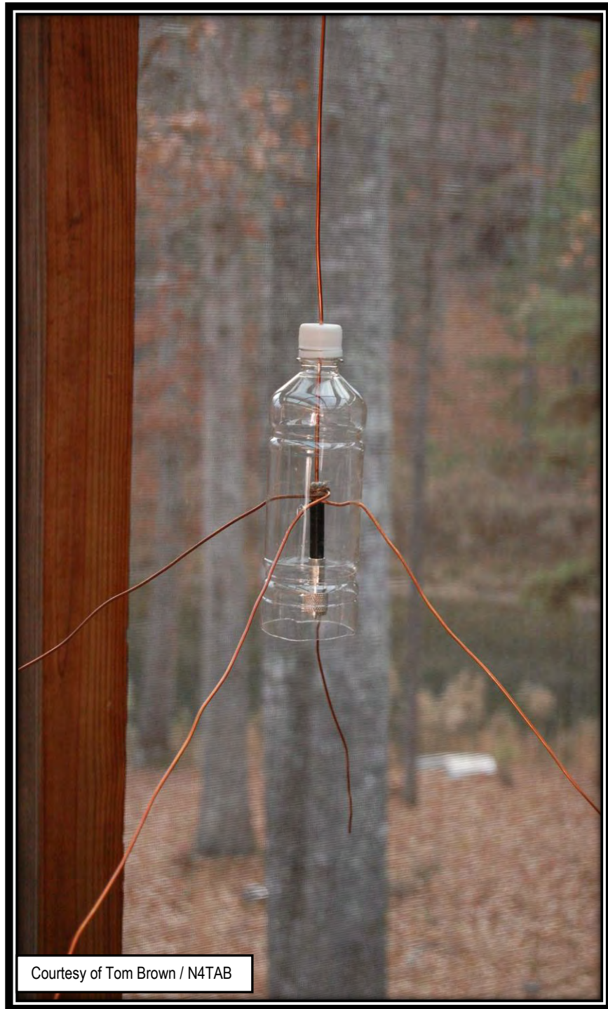
Figure 2. Example of VHF Ground Plane Antenna
