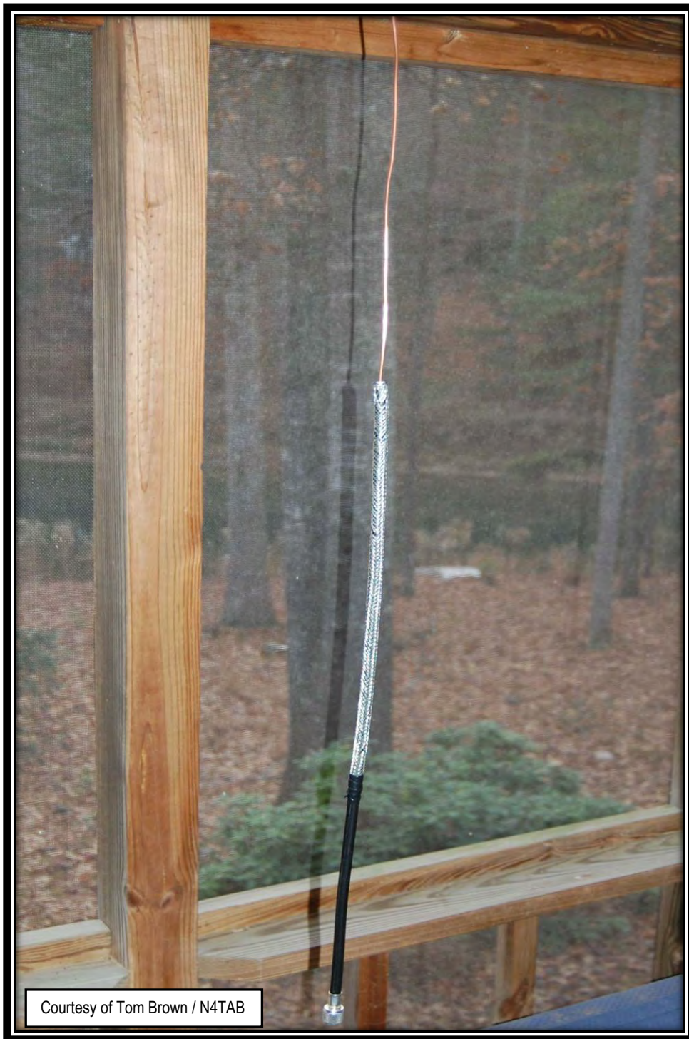
Figure 4. Example of VHF Coaxial Sleeve Antenna
