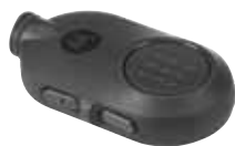
NNTN8127 Wireless Push-to-Talk Pod. This pod is compatible with any wireless Bluetooth headset and provides wireless Push-to-Talk functionality. Also comes with a micro USB charger.
