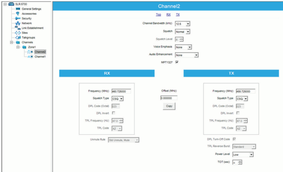
Figure 79: CPS Configuration for TSCC03 Channel Controller (2 of 2)
