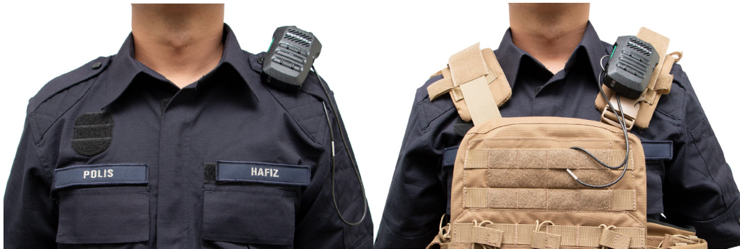
Figure 3: Recommended Wearing Positions—Using Tethering Kit Accessory with Velcro pad
