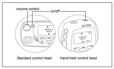
When the radio is first turned on, the red, green, and orange LEDs flash briefly, and the radio gives two short beeps. A brief message may appear on the display.
